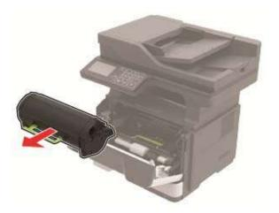
**3** Remove the used imaging unit.
