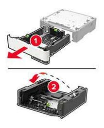
**5** Remove the used pick roller assembly.
